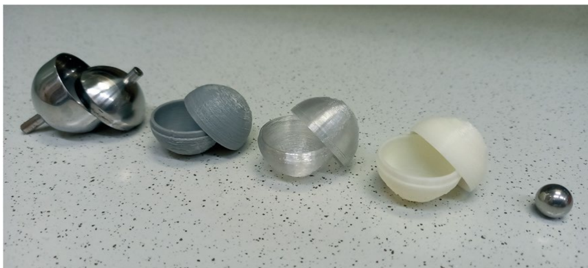
Fig. 1. The steel jar of a vibrational mill (NARVA Vibrator DDRGM9458, 50 Hz) and the 3D-printed polymer inserts for it (from left to right: PLA, PETG and ABS), as well as a steel ball (9.5 mm diameter, 3.5 g)
